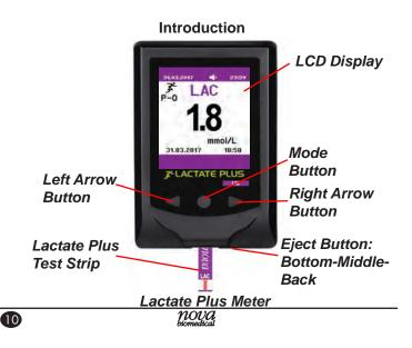
The Lactate Plus Meter is a hand-held testing device that measures lactate (LAC) in whole blood. The test strip is touched to a drop of blood to initiate the test process.
